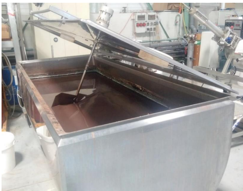
Figure 16: Vinasse storage tank
